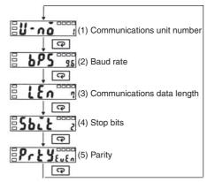
Align each communications setting with the settings on the personal computer or other communications device.
