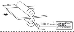
Note: The count will become incorrect if the prescale value is not set correctly. Check the setting to be sure it is correct.
