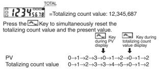
Refer to *Input/Output Mode Settings* on page 20 for information on totalizing counter operation.
