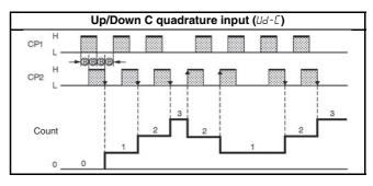
Note: 1. (A) indicates the minimum signal width and (B) requires at least 1/2 the minimum signal width. If these conditions are not met, a counting error (+1 or -1) may occur.
