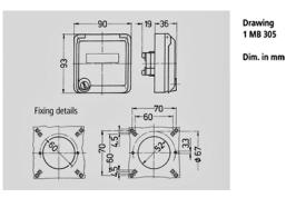
for TKM type KDMF, also suited for data modules of Telegärtner (AMJ 45 Up/O, Cat.6a) and Nexans (LANmark-6 Snap-in Connector with jumper ring Modular Outlet 50)
