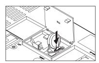
(5) Disconnect the cable connector of the backlight from the GOT side connector.
